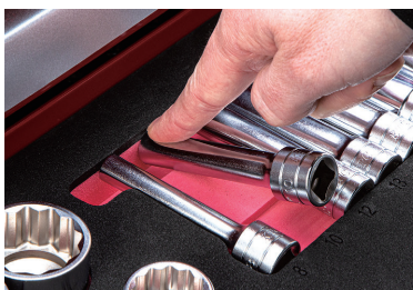
A push-up system is used whereby one side of the tool is pushed and the other side comes up. Laser-engraved size markings are also provided for quick access to the tool you need.
