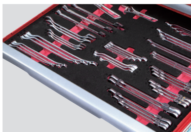
Layout that considered for frequently used tools. Frequently used tools are placed in front of the drawers. This reduces the time to take them out.
