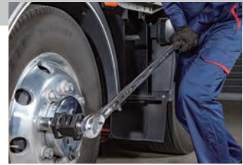
Tightening of bolts and nuts
