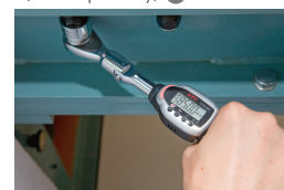
Head can be flipped over for use
