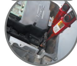
Voltage measurement required before work is specified in the vehicle manufacturer's maintenance instructions.
