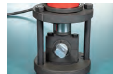
(2) Compression of cracked bushings
