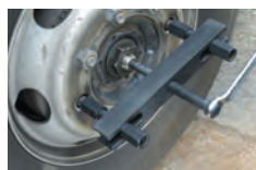
Front wheel hub extraction
