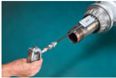
Nozzle adapter for easy injection without removing bearings
