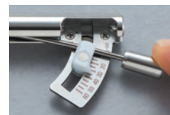
Needle to reduce reading errors
