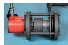
(3) Press fitting of bushing
