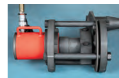
(3) Press-fit the split bushings
