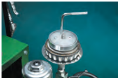
Removed bearings can be greased by setting them in the cone
