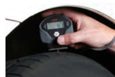
Measuring tire grooves and filling out inspection records
