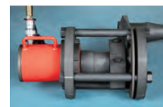
(3) Press-fit the split bushings
