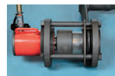
(3) Press fitting of bushing
