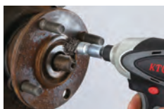
For cleaning and rust removal around automobile axle hubs
