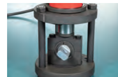
(2) Compression of cracked bushings
