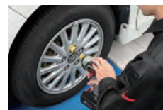
Tire installation (temporary tightening)
