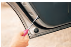
The clip can be easily removed by leverage without damaging the interior lining.
