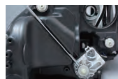
The intermediate shaft is 5 mm in diameter, allowing smooth access even in narrow service holes.
