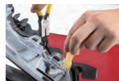
Disassembly of headlamp lenses
