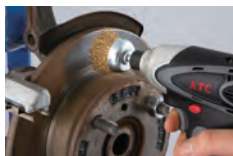
For cleaning and rust removal from brake rotor surfaces
