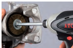
For cleaning O-ring grooves of brake calipers
