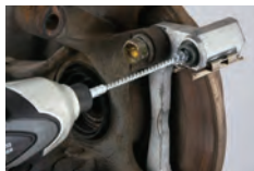
To clean sliding pin holes in brake calipers
