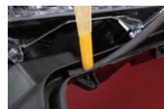
Assembling the gasket to the housing
